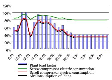
The graph shows the relationship of daily air consumption of the plant and the corresponding electrical consumption of the compressor. When air consumption fluctuates the variable pump drive control logic is much more efficient.
