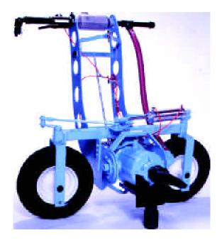
The **Sidewinder** is the most versatile **POGO**, designed to open gates with both the stationary style and rolling style drive knuckles. Unique to this model are its pneumatic controls (drive direction/wheel rotation). With the touch of a switch the pneumatic wheels rotate 90° to allow the machine to roll with the gate.
