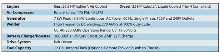
Air N Arc® 300 Gas Unit Dimensions: Foot Print (In.): 47.1L x 21.5W x 30.9H With Fittings (In.): 47.1L x 24.6W x 30.9H Dry Weight (Lbs.): 700
