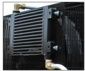
Air cooled after cooler on Elite unit
