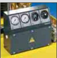
Our standard instrument panel contains gauges for air temperature, oil pressure, inlet air pressure, and discharge air pressure.
