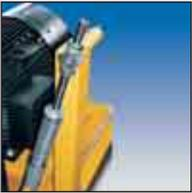
V-belt drive with an easily accessible automatic tensioning device provides optimum power transfer and long belt life.
