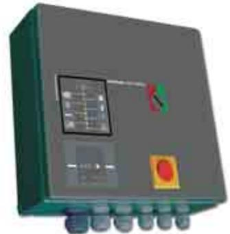
Kaeser offers an enhanced starter control panel to monitor and regulate booster operation. Units from 3 to 25 hp are 230/460 V with direct on-line start. Units 30 hp and larger are 460 V with wye-delta start (consult factory for other voltages). The starter is designed to be wall-mounted.
