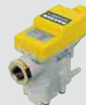
All AirCenters come standard with one Eco-Drain in the dryer (and on the receiver with the optional Clean Air Treatment Package). The Eco-Drain automatically removes liquid contaminants from the tank without wasting valuable compressed air.
