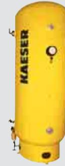
Receiver tanks play a vital role in your air system, and that is why every AirCenter has one. They separate bulk liquids from the air stream, reduce compressor cycling and store air for intermittent volume demands without a drop in system pressure. AirCenter tanks are ASME coded and include a properly sized safety relief valve and pressure gauge.
