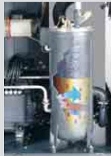
high-efficiency separation system. Most of the cooling fluid is initially separated from the air by centrifugal force in the separator tank. Any remaining fluid is separated by a 2-stage
