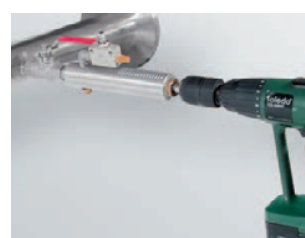
Drill under pressure with the CS drilling jig
